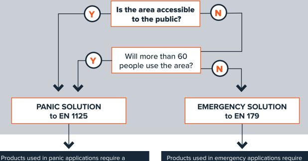
Products used in panic applications require a device that covers at least 60% of the width of the door such as cross bars or touch bars.
